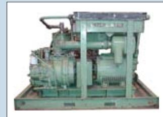
Step 4: Air compressor is fully tested and ready for paint.
