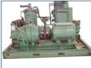
Step 3: Air compressor is assembled from rebuilt components.
